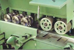
Effortless feeding of thin and difficult material up to 120m/min, guaranteed with top and bottom feed rolls throughout the machine.
