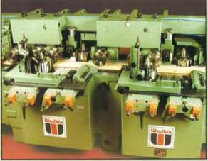
Extended cutter life and improved finish with the option of prerelieving heads. Side head bedplates are easily adjustable laterally for varying cutting circles.
